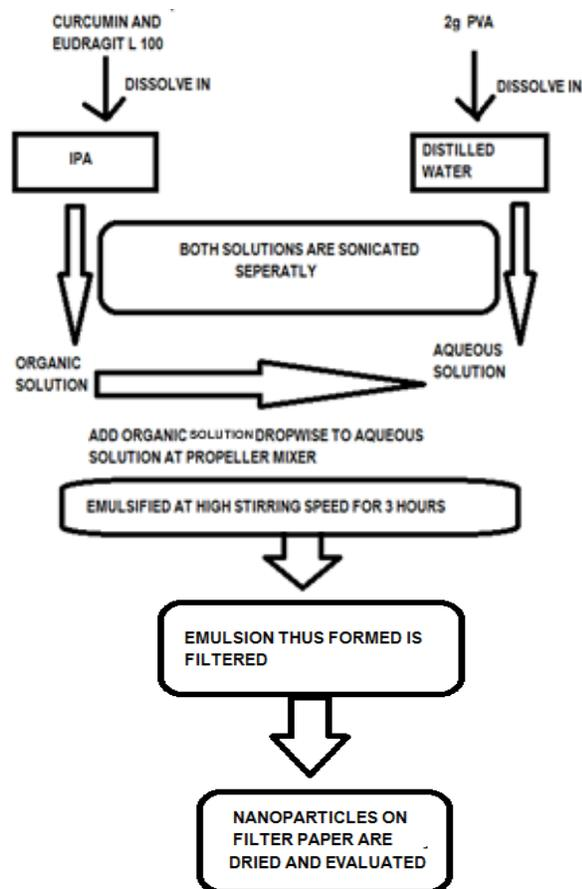
Figure 1: Schematic representation of nanoparticles containing curcumin and Eudragit L-100 as polymer.
